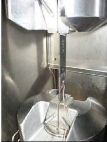
Figure 2: Open-hole tensile test setup
