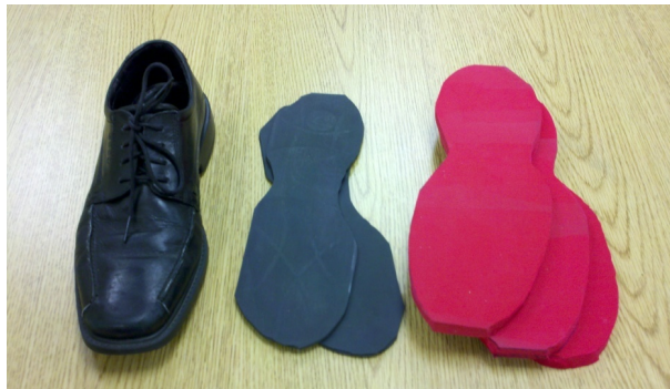
Figure 4. Shoe (left), 0.125 in rubber platform (center), 0.50 in foam platform (right).
