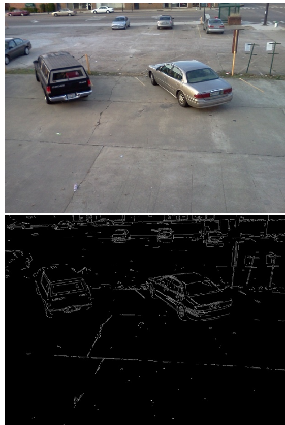
Figure 2. Snapshot before and after being processed with edge detection
